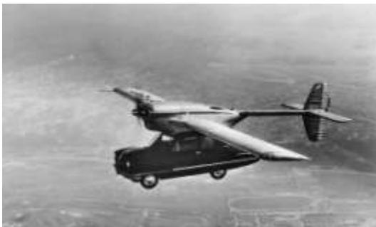
Consolidated Vultee Aircraft (yes, the same folks that gave us the B-36 bomber with 6 radial and 4 turbojet engines) developed the ConVairCar Model 118 flying car in this same time period. Like Mr. Fulton's creation, lots of stuff was left at the airport before one could head out on the town. The ConVairCar
