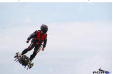
jet engines capable of providing controlled, directional thrust. The pilot straps his feet onto the board and is able to hover, spin, climb and descend on command with simple control inputs to the motors. High speed passes are even possible at 90 mph speeds. Here is the video clip I am referring to:
